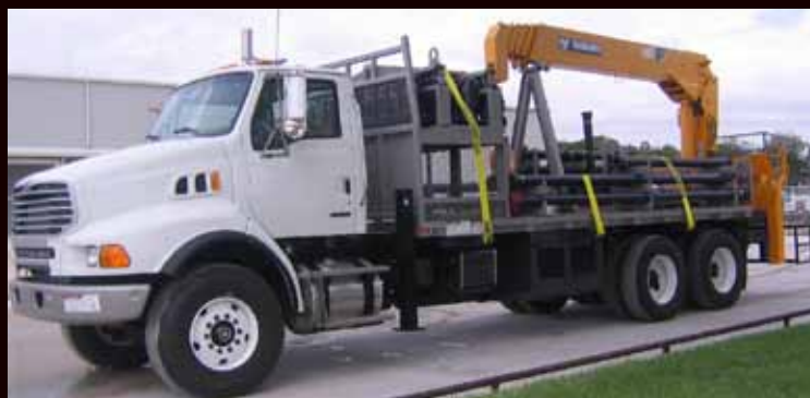
Crane Truck 10-Ton with custom Swivel & Flowline racks
