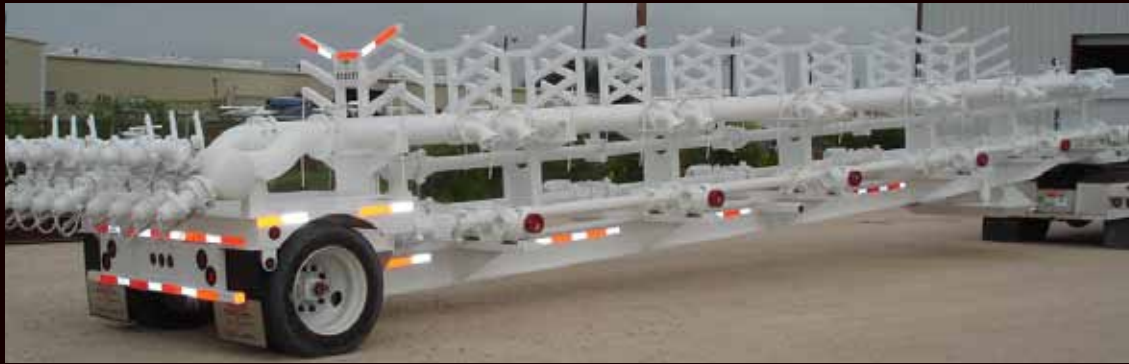
12 Pump Unit - 4"1502 Tees with 3" Valves 15,000psi
